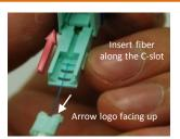
② Insert the cleaved fiber slowly into the rear of connector until connection is made.
