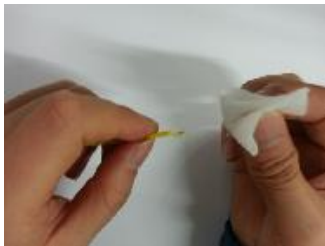
7/ Clean the stripped fiber with alcohol wipe to remove any debris.
