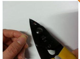
2b/ If for 250 or 900µm cable, strip off around 35mm coating, then jump to point 6.
