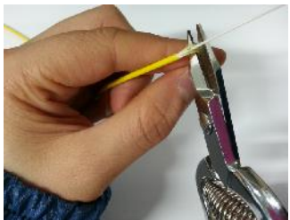
3/ Cut Kevlar to the length of 4mm.
