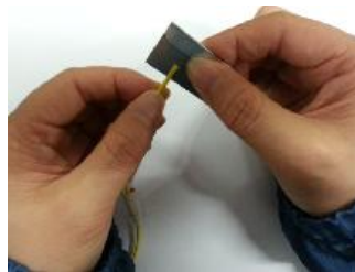
5/ Split the cable jacket by 6mm with a blade.
