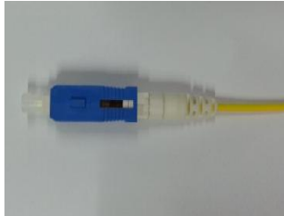
6/ Release wedge clip and termination is done.
