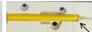
a/ For 2mm or 3mm cable, set the cable edge at above shown point.
